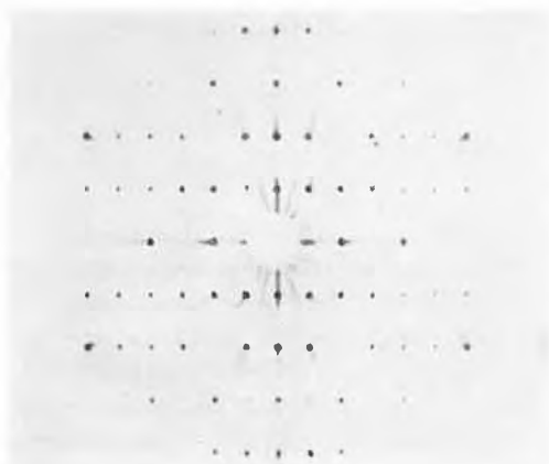
Figure 1. A layer of the diffraction pattern produced by a crystal of acenaphthene
