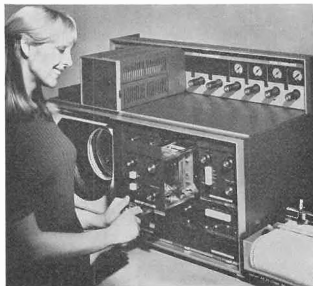
Fig. 2. The Pye Unicam GCV gas chromatograph is designed for diverse uses. Its detector oven, in which three different detector systems can be operated simultaneously, is especially significant (Pye Unicams Ltd., York Street, Cambridge CB1 2PX, England)
