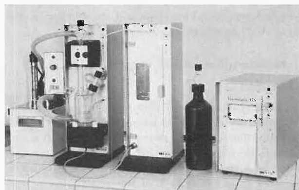
Fig. 2: High precision automatic viscometer VISCOMATIC M.S. FICA. From the left to right: thermostatic bath, actual viscometer, programmed dilutor, printer.
