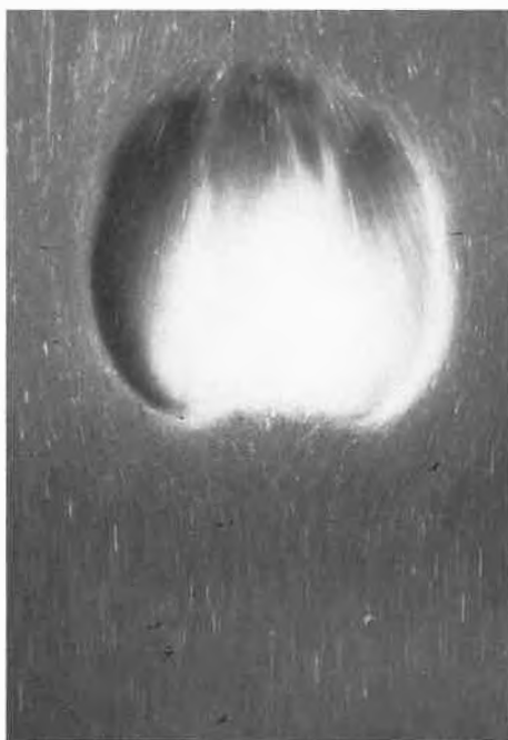
Fig. 2: An isolated bubble rising through a two-dimensional bed.
