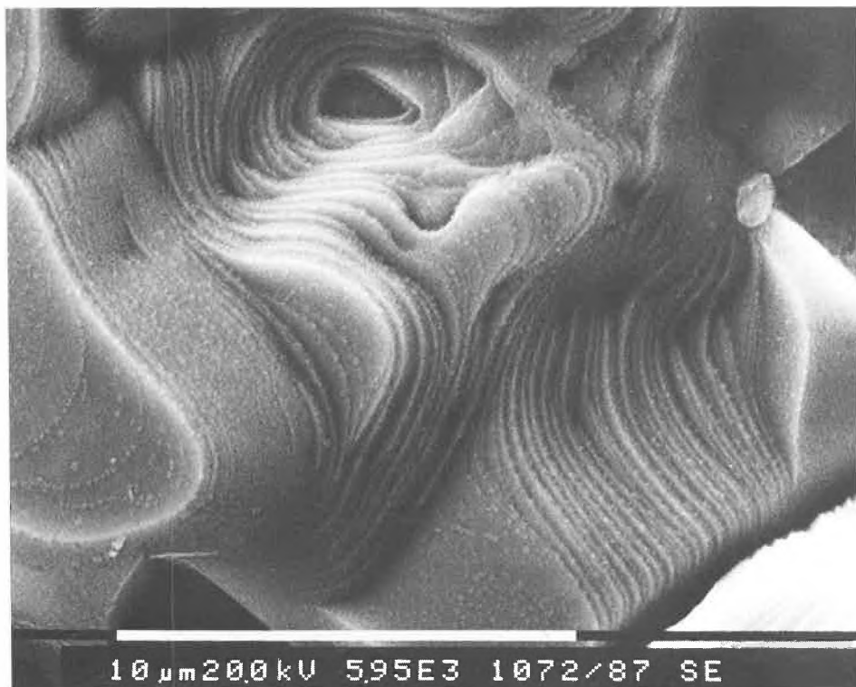
Fig. 5. Scanning electron microscopy (SEM) photographs of EuBa_2Cu_3O_{7-x} , a 94 K superconductor. The material is composed of grains of different size which are only loosely connected (above). The grains show a layered structure which is typical for high- T_c oxides (below).
