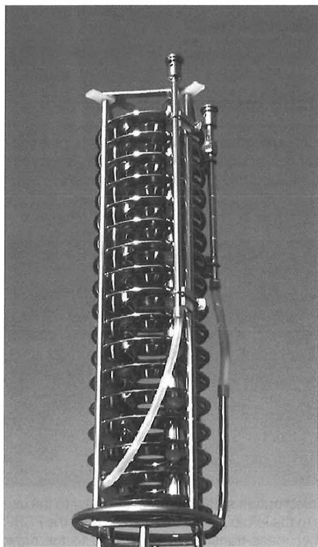
Fig. 5. The Air-Trap-Aeration unit as it is used for the aeration of hybridoma cells in a standard 25 litre bioreactor.
