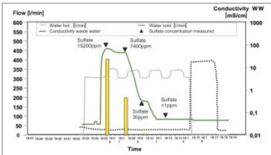
Fig. 1. On-line measurements of water consumption (hot and cold) and wastewater quality (conductivity and sulfate concentration) were used to improve a batch washing process.
