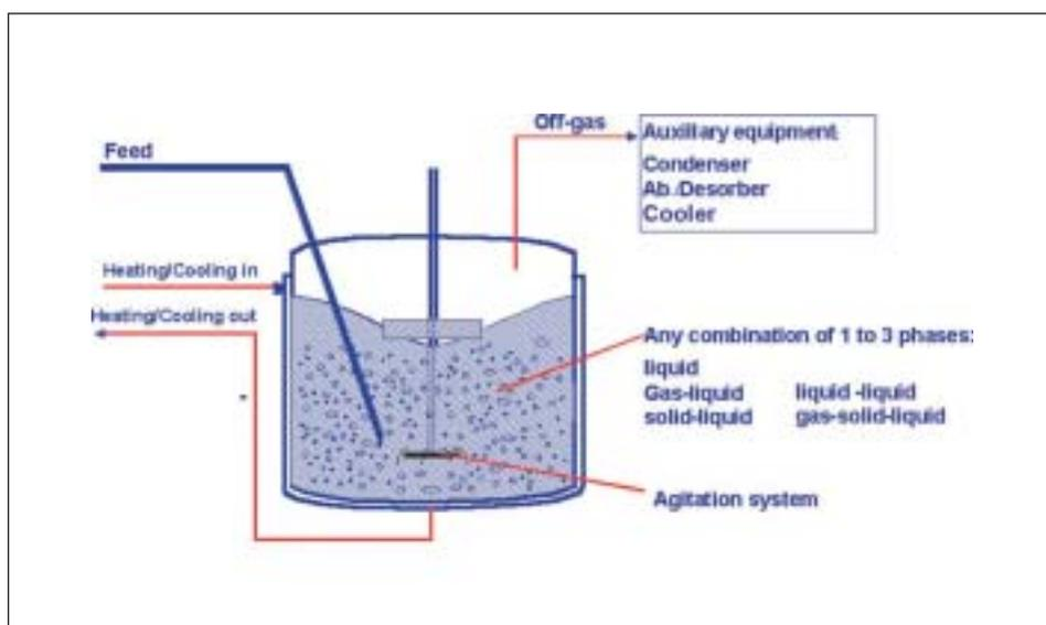
Fig. 8. Schematic of a typical semi-batch reactor
