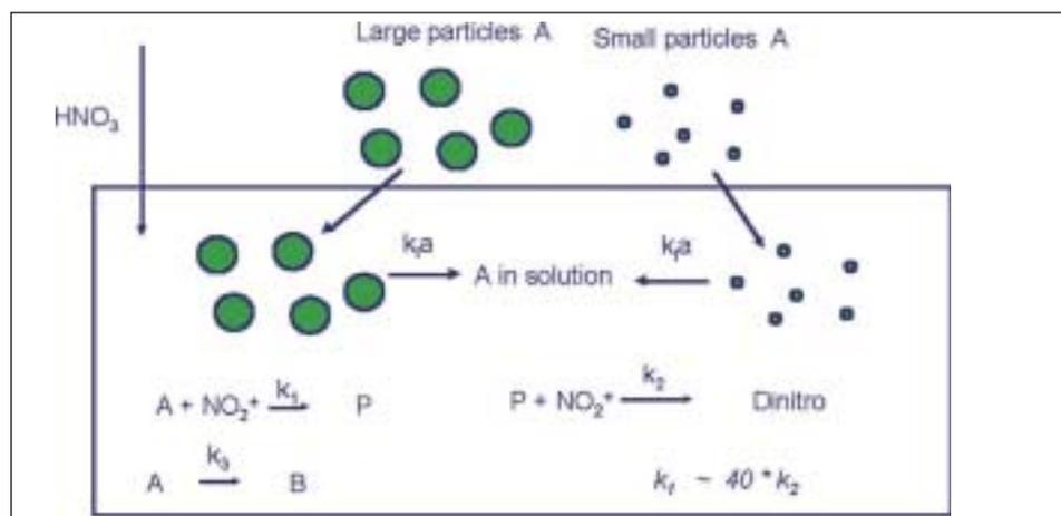
Fig. 11. Process scheme for nitration example
