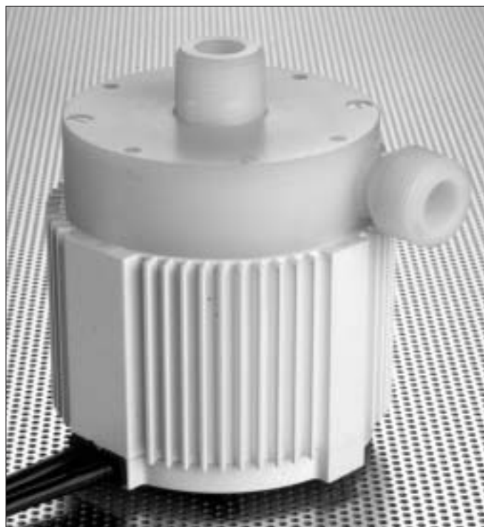
Fig. 5. Bearingless canned-motor pump for the semiconductor industry with a high purity PVDF pump and chemically resistant motor housing (ECTFE coated).
