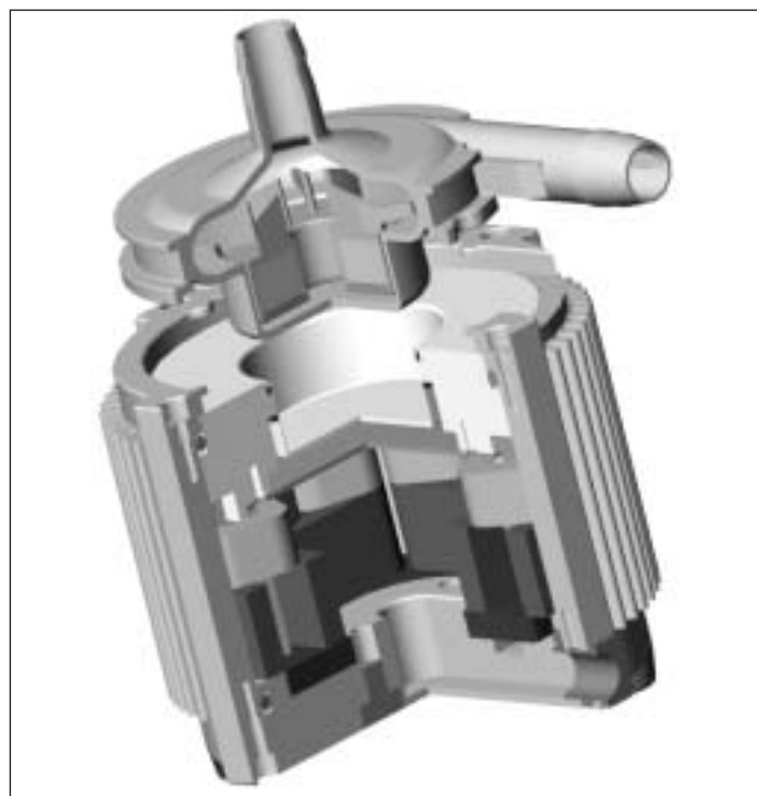
Fig. 3. Design of a bearingless canned-motor pump with disposable pump.
