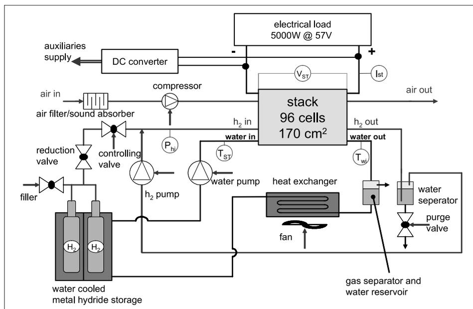
Fig. 13. Scheme of the SAM liquid-cooled fuel cell system
