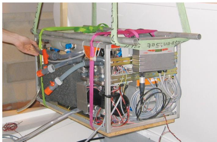
Fig. 16. 3 kW, water-cooled, fully automated fuel cell system is mounted to vessel. Volume 170 l, weight 70 kg.
