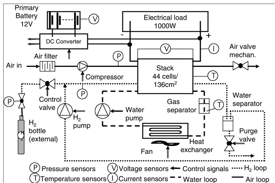
Fig. 4. Scheme of the liquid-cooled PowerPac fuel cell system
