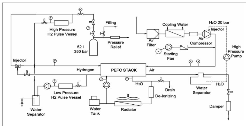
Fig. 19. Schematic of liquid-cooled fuel cell system, with air humidification through water injection into compressor
