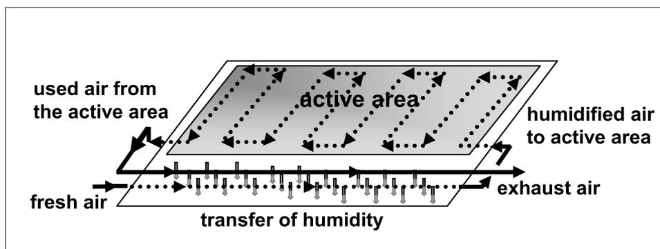
Fig. 5. Concept of internal process air humidification by transfer of humidity through a separate membrane section from the used air to the fresh air within each cell
