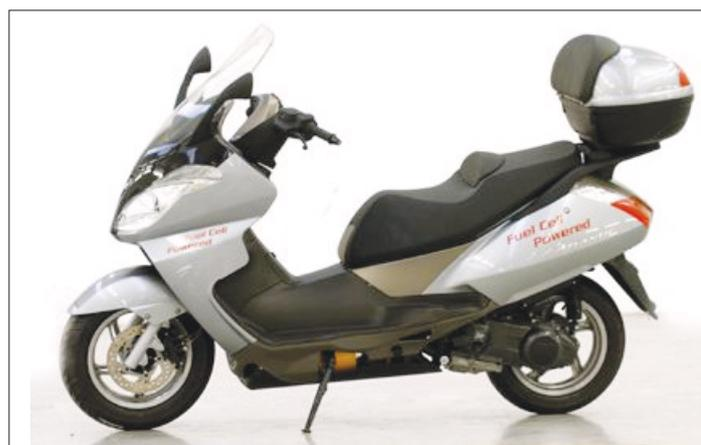
Fig. 11. Aprilia Atlantic Zero Scooter equipped with MES-DEA 6.0 kW Fuel Cell System. Details see text
