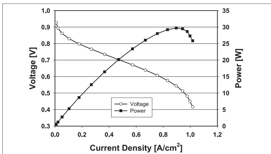
Fig. 8. Current/voltage and current/power curves of a 61 cm<sup>2</sup> single cell at 62 °C; Hydrogen pressure 1.4–1.5 bar<sub>a</sub> (dead end); air near ambient pressure, stoich. 2.5–4.5. No gas humidification.
