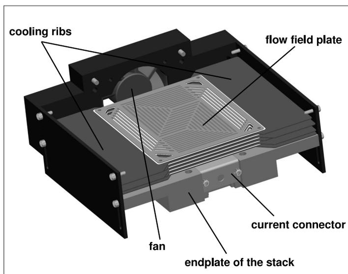
Fig. 2. CAD model of inside view into a 5-cell stack including cooling fan and housing
