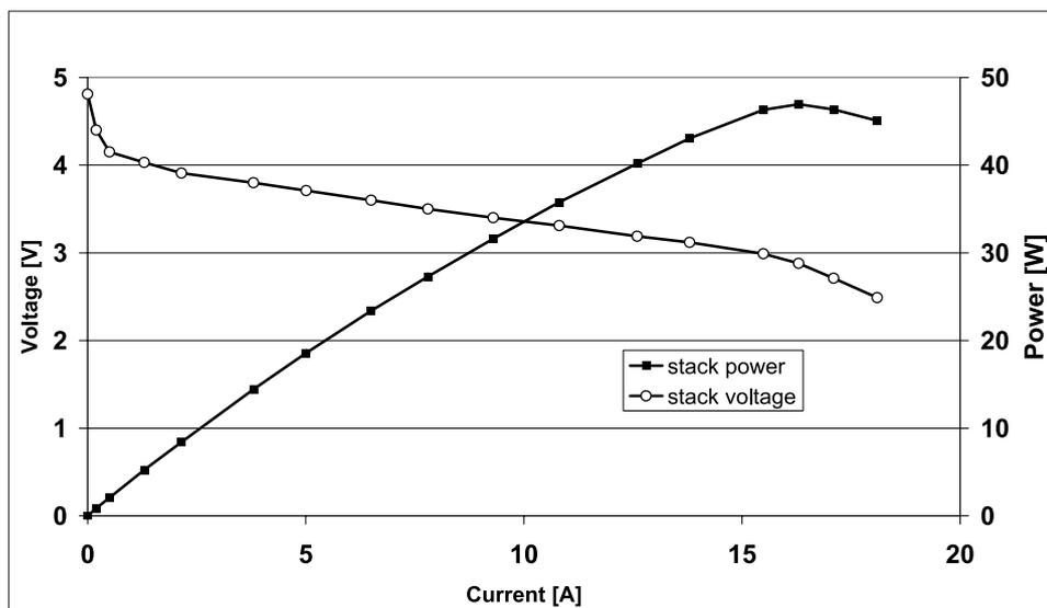
Fig. 3. Current voltage and current power curve of a 5-cell stack at 50 °C; both gases near ambient pressure
