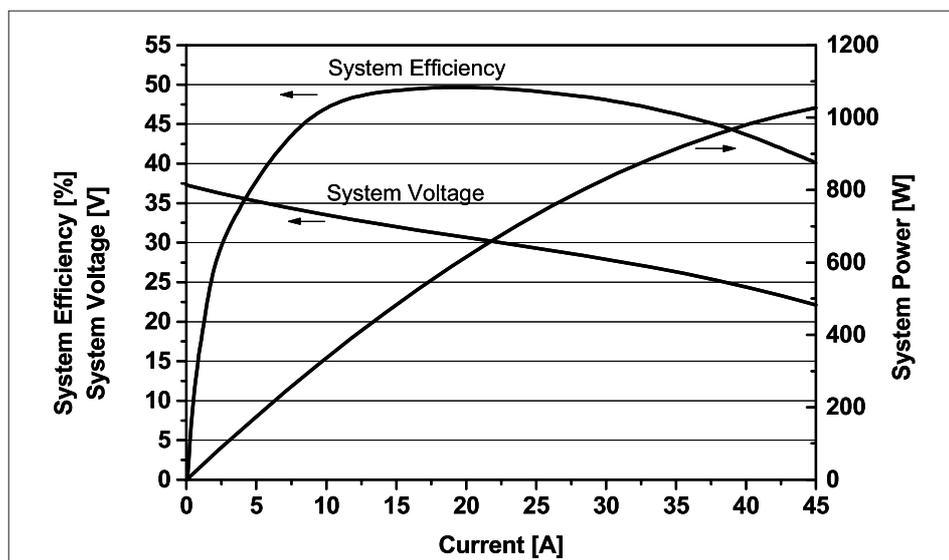
Fig. 7. Current/efficiency, current/voltage and current/power curves for the PowerPac system at an operating temperature of 65 °C
