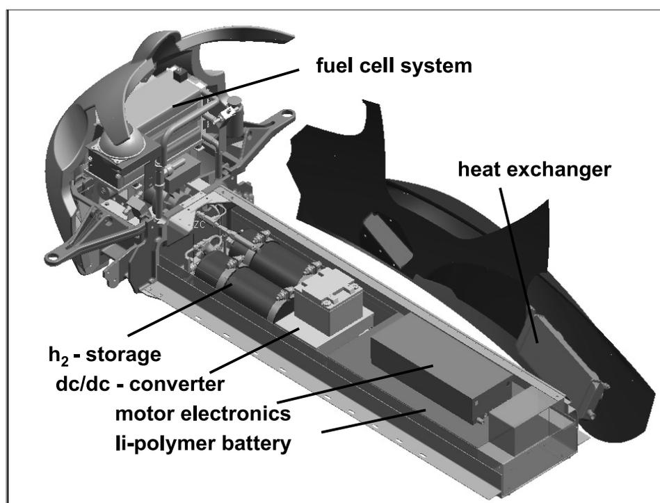
Fig. 14. CAD model showing the positioning of the system components in the SAM vehicle
