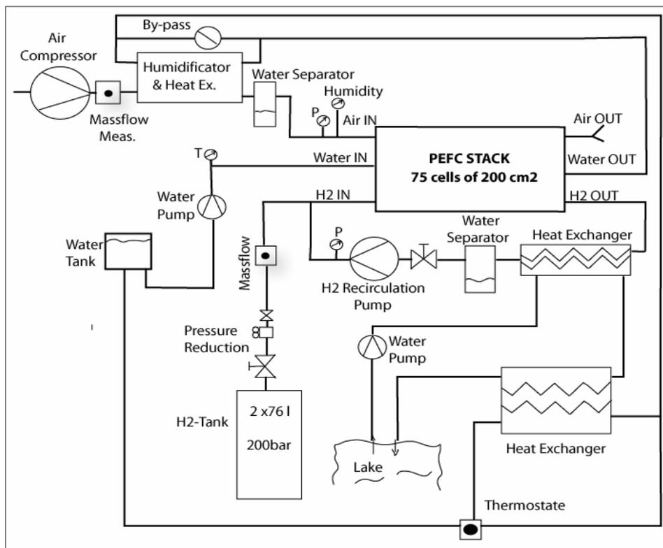
Fig. 15. Scheme of lake-water-cooled 3 kW fuel cell system
