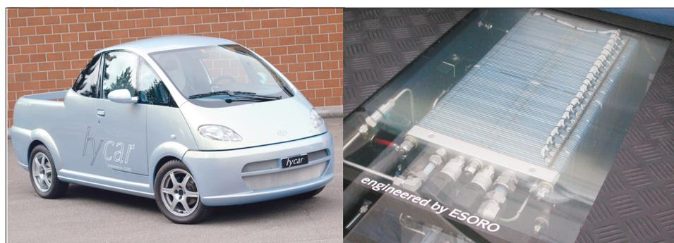
Fig. 22. Left: the concept car HyCar; right: its visible fuel cell system
