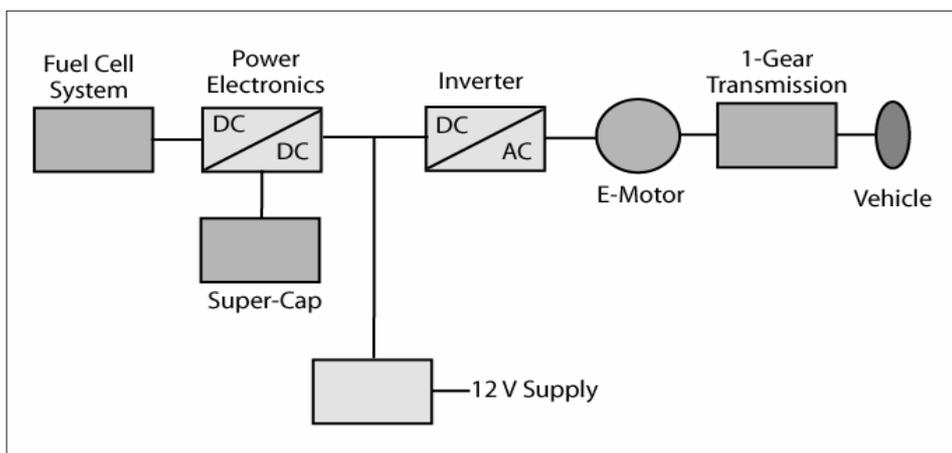
Fig. 18. Configuration of the powertrain of the Hy.Power PEMFC-hybrid passenger car
