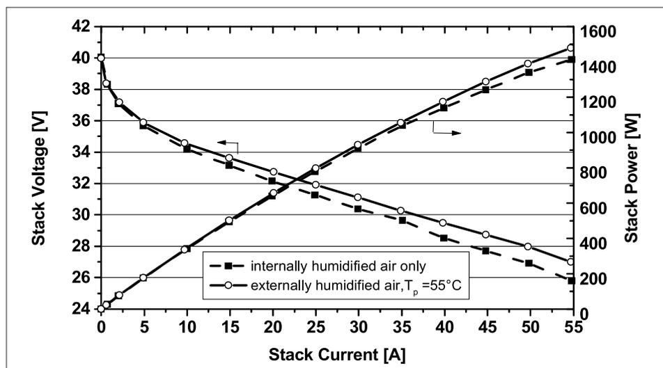
Fig. 6. Current/voltage and current/power curves of the PowerPac stack at 65 °C with and without external humidification of the process air. Hydrogen: stoich. = 1.2, pressure 1.3 bar<sub>a</sub>; air: stoich. = 1.8, pressure 1.4 bar<sub>a</sub>.
