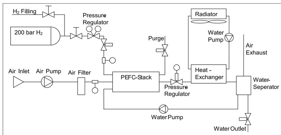
Fig. 23. HyCar's fuel cell system with Nuvera's direct injection cooling (combined cooling and humidification water circuit in the stack)
