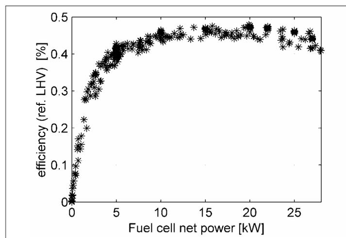
Fig. 20. Current-based system efficiency of the Hy.Power car during operation
