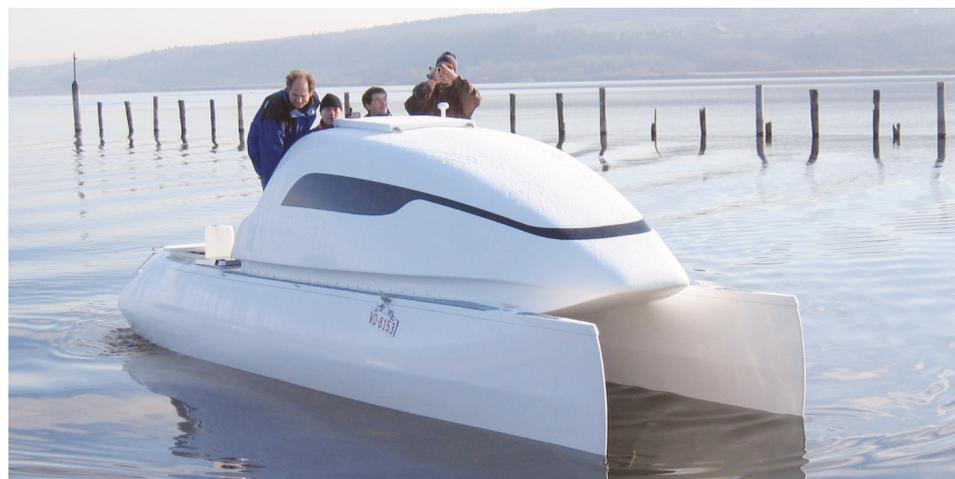
Fig. 17. Electric boat Hydroxy3000 for six passengers, with 3 kW PEMFC/battery hybrid electric propulsion system, speed 12–18 km/h, size 7m x 2,5m, weight 1300 kg
