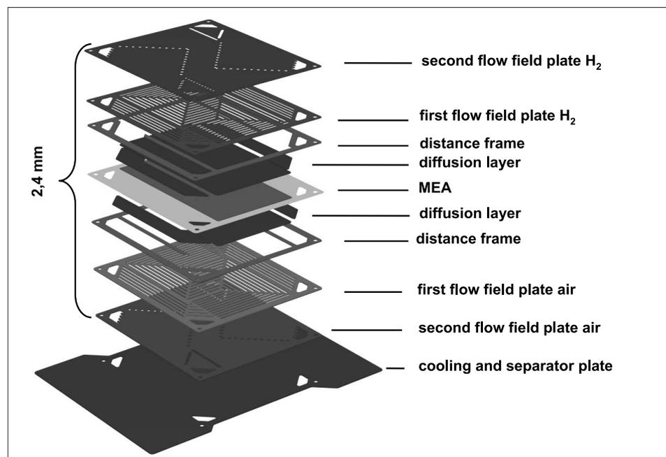
Fig. 1. Explosion view of the complete cell, showing the eight layers of a stack repetition unit
