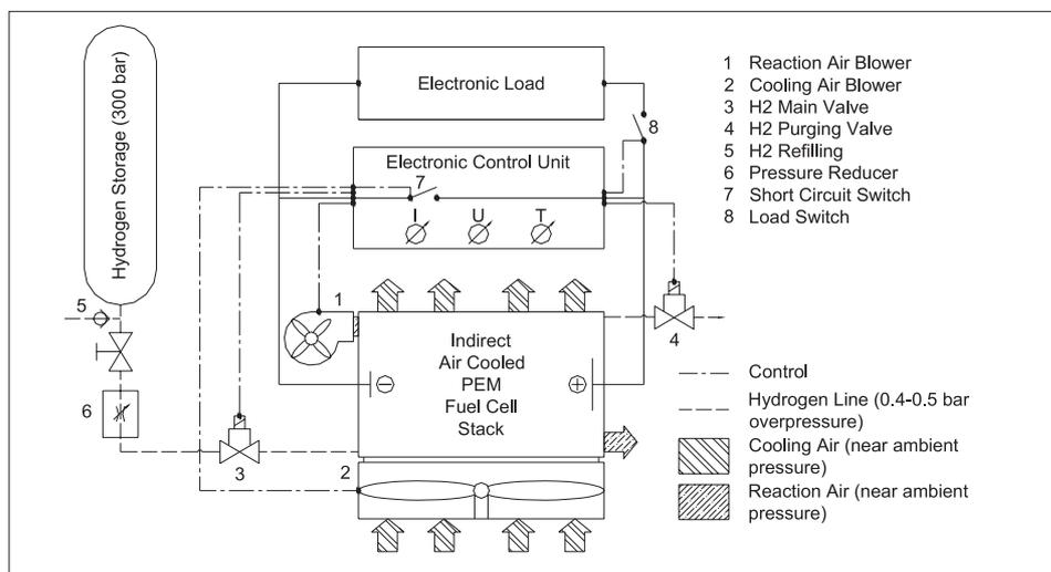
Fig. 10. Scheme of air-cooled fuel cell system for light mobile applications
