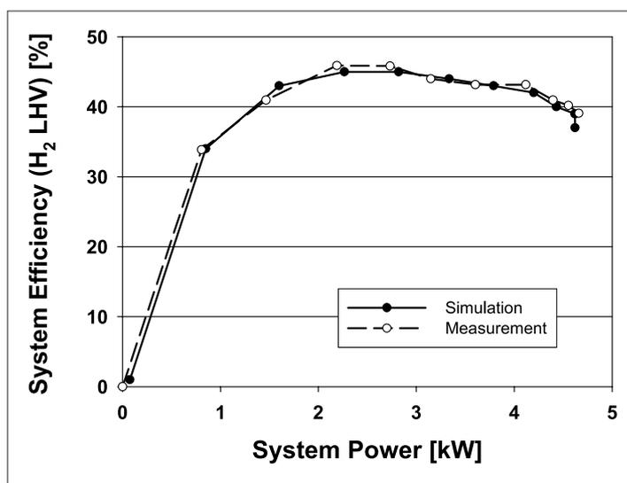
Fig. 24. Simulated and measured current based system efficiency of the HyCar fuel cell system
