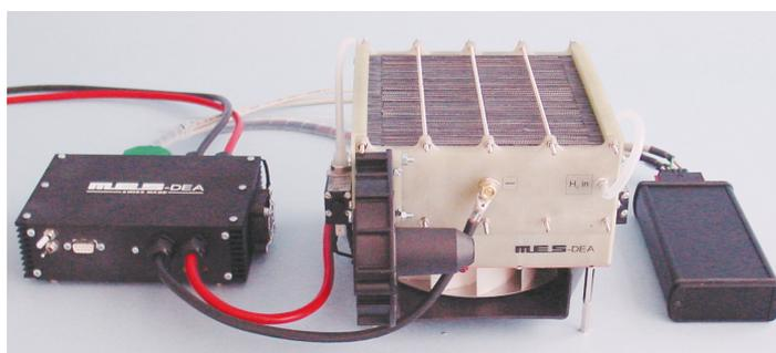
Fig. 9. 1.0 kW Fuel cell system with cooling blower control unit (right box) and electronic control unit (left box). Cooling blower below stack and process air blower on front end
