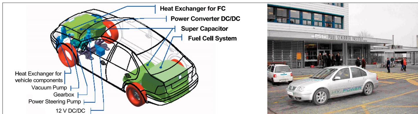
Fig. 21. Packaging of the adapted systems for the fuel cell power train in the VW Bora Hy.Power (left), and vehicle in operation (right)
