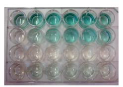
Colorimetric arsenic bioassay. Cells produce beta-galactosidase in response to the presence of arsenite in the medium. Image shows different cell lines (in rows) with varying response kinetics. Arsenite concentrations (left to right): 0, 0.1, 0.2, 0.5, 1.0 and 2.0  $\mu M$ . Incubation time 3 h at 35 °C. Image courtesy: Jan R. van der Meer.
