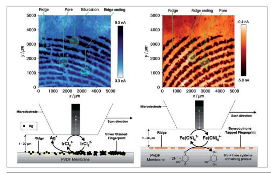
Top: Constant height SECM images of a fingerprint developed by silver staining (left) or benzoquinone tagging (right). Bottom: Schematic representation of the detection principle of silver nanoparticles containing fingerprints (left) and benzoquinone-tagged fingerprints (right).
