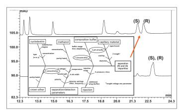
Fishbone diagram for a capillary electrophoresis method. Proper control of critical method variables and critical interactions will ensure proper method performance: Crown ether concentration increase leads to separation of (S) and (R) impurity.
