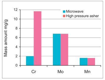
Extraction efficiency of the microwave method vs. the high pressure asher (HPA). It is obvious that Cr with the microwave method is 6 times lower then with the HPA method. The cause is the formation of chromiumcarbide (CrC) with the microwave method.
