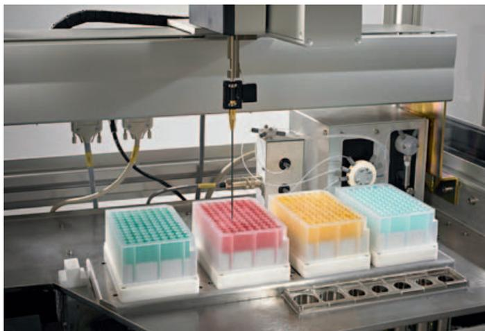
Tecan's Cavro® Omni Robot has been incorporated into Applied Photophysics' new protein discovery solution, the Chirascan™-plus CD Spectrometer. This newly created system combines Tecan's precise and reliable sample handling with excellent measurement reproducibility, opening up a wide range of circular dichroism (CD) applications for the first time.
