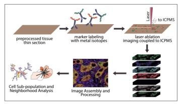
Workflow for imaging mass cytometry, based on mass cytometry and laser ablation ICPMS imaging.
