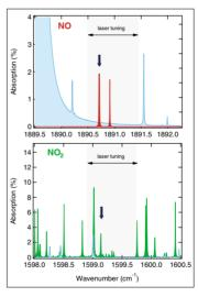
Simulated transmission spectrum of  $NO_2$  (green), NO (red) and water vapor (blue), and the tuning range of the DW-QCL. The targeted absorption peaks are indicated with a blue arrow.
