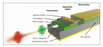
Schematic drawing of the dual-wavelength laser. The laser is approximately 200  $\mu m$  wide and 5 mm long. It emits at 5.26  $\mu m$  (1900 cm<sup>-1</sup>) and 6.25  $\mu m$  (1600 cm<sup>-1</sup>) as indicated by the two-colored beam.
