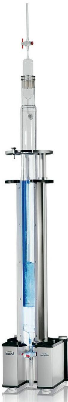
The KRÜSS Ross Miles Foam Analyzer – RMFA for electronic foamability measurements to ASTM D 1173
