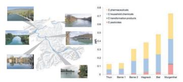
Micropollutants in the river Aare at six downstream measuring points with increasing population density and intensity of agricultural activities in the catchment area. The concentrations are not critical for water organisms, but the load at Murgenthal (top right) of 16.2 kg micropollutants per day is very high.
