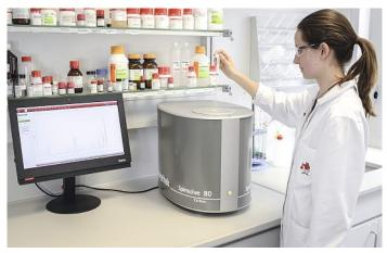
be more than 10.000 larger that the signals of interest, the suppression method offered with the Spinsolve also includes carbon decoupling to eliminate the signal of the carbon satellites of the main solvent signals.
