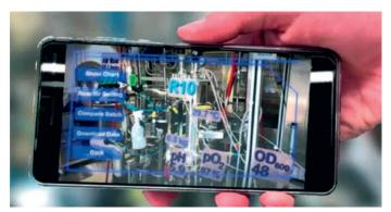
Fig. 8. Concept for AR visualization of bioprocess data on mobile devices. In context-sensitive displays, the most relevant key information is directly accessible.
