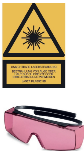
Fig. 3. OTG safety glasses suitable for a 785 nm Laser.
