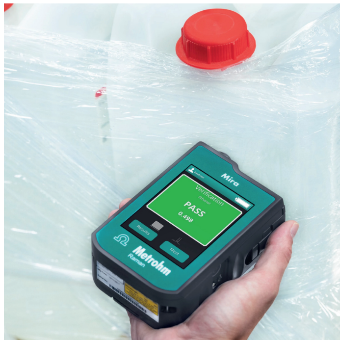
Fig. 4. Sample identification with a handheld Raman spectrometer. In this case, the identification of a liquid is done through packaging material.
