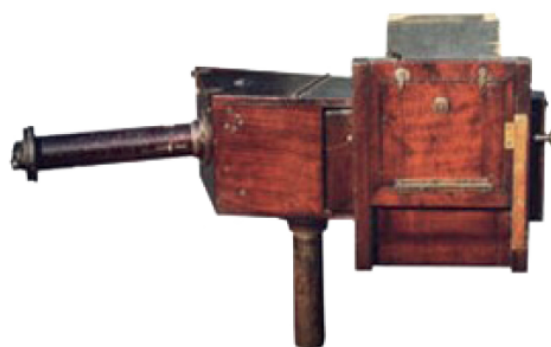
Fig. 1. C. V. Raman’s instrument to confirm his hypothesis of inelastic scattering, which was later named after him: Raman spectroscopy.
