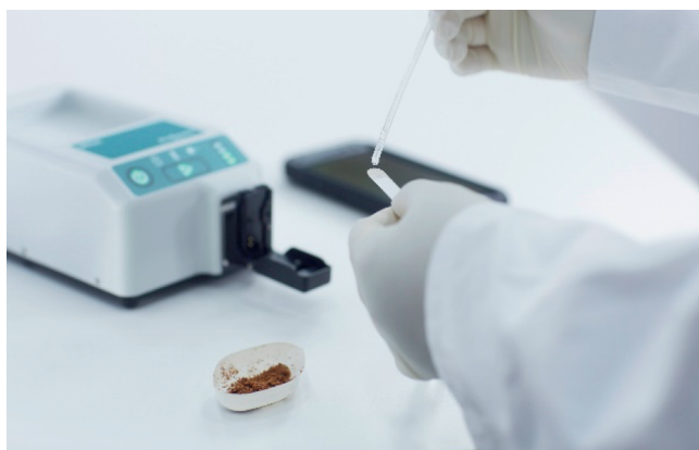
Fig. 9. Sample preparation on a SERS Strip. A dedicated SERS instrument with an open SERS attachment is in the background.
