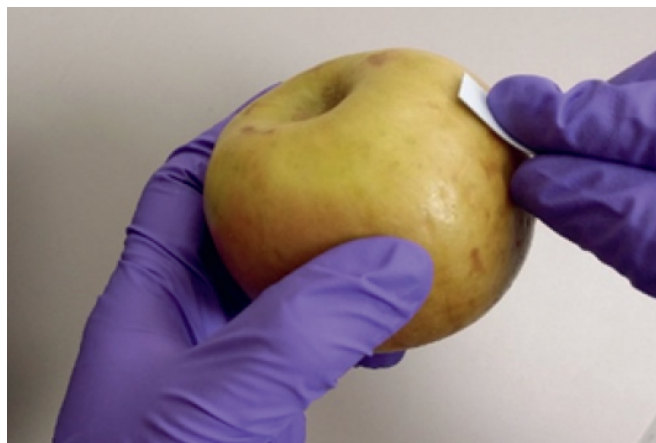
Fig. 10. Sample preparation with a SERS Strip for Thiram: rub the strip on the apple surface.
