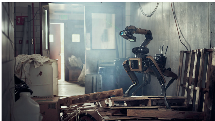
Fig. 2. Handheld Raman (MIRA XTR) mounted on a robotic device to enter a danger zone. A zoom lens allows for sample identification from a 2 m distance to the instrument. Handheld Raman devices can also be mounted on flying drones for chemical identification.
