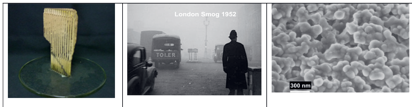
Fig. 1. Left: Fragment of a DB particulate filter from the 1988 damage series. Source VERT; Centre: London SMOG 1952; Right: Soot particles in the lungs of London SMOG victims, source Ref. [3].
