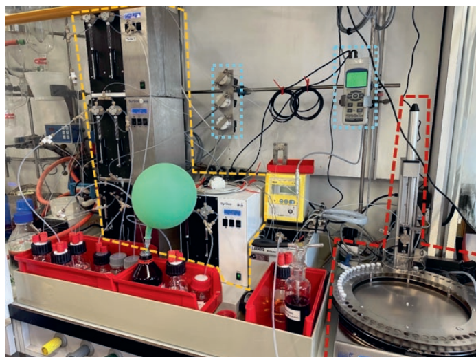
Fig. 4. First-generation standard setup comprising pumps (highlighted in orange), pressure and temperature sensors (highlighted in blue), pressure regulators, and a sampler (highlighted in red). Equipment is controlled by a DCS (Hitec Zang GmbH), itself driven by a Python script.
