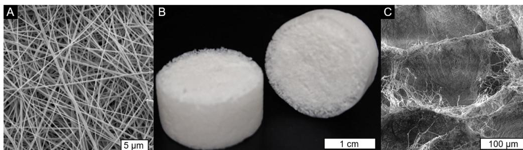
**Figure 1.** (A) Chitosan/PEO nanofibers with diameter of  $309 \pm 56 \text{ nm}$ ; (B) chitosan nanofiber sponges with their hierarchical open pore architecture shown in a cross section image (C).
