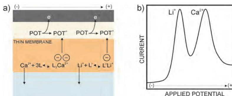
**Fig. 1a)** Scheme of the electrochemical process (L=calcium ionophore and L'=lithium ionophore). **b)** Voltammograms obtained for equimolar concentrations of lithium and calcium.
