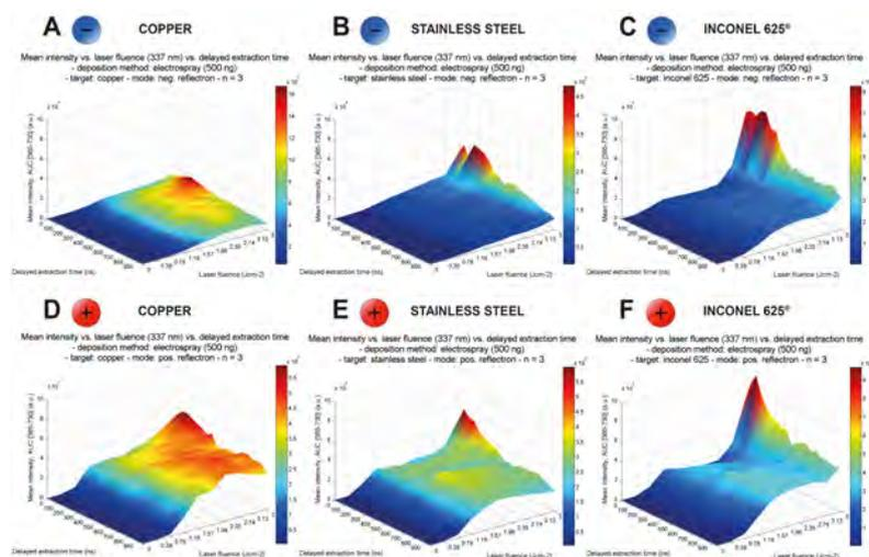
Figure 1. Ion yield vs. extraction delay time and laser fluence in negative reflection mode for: A) copper, B) stainless steel, used as standard (MALDI) target plate material and C) inconel 625<sup>®</sup> (Ni1/Cr22/Mo9/Fe5). Ion yield vs. extraction delay time and laser fluence in positive reflection mode for: D) copper, E) stainless steel F) inconel 625<sup>®</sup>. Note: each color bar ranges from zero to the maximum ion yield measured for the corresponding graph.
