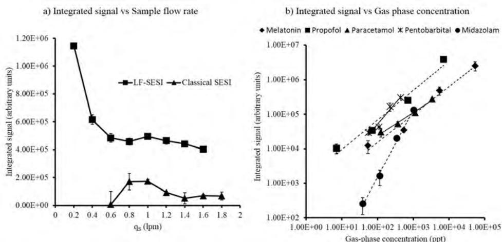
Figure 1. a) Experimental performance of the LF-SESI and the Classical SESI varying N<sub>2</sub> sample flow rate; b) Examples of drugs detected with the Universal LF-SESI
