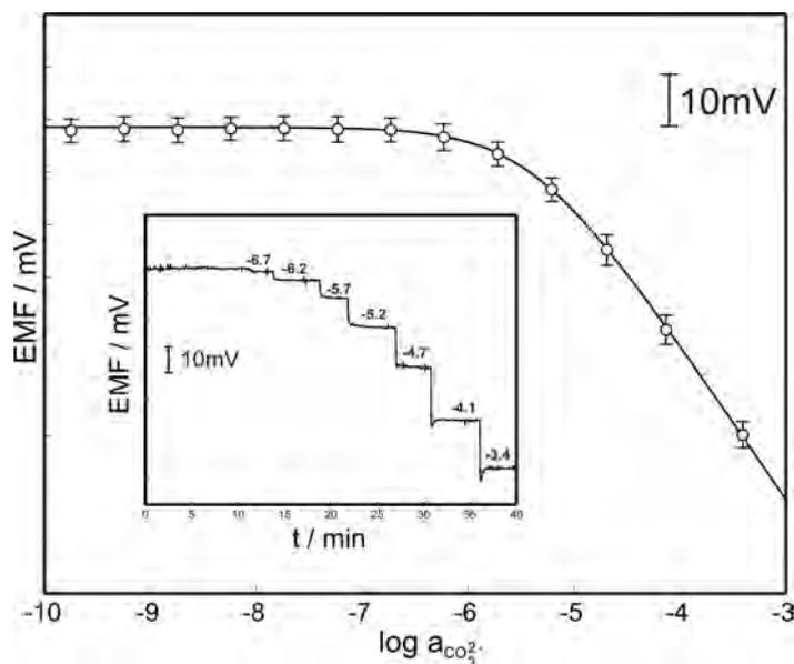
Fig.1. Calibration curve of the all-solid-state carbonate electrode
