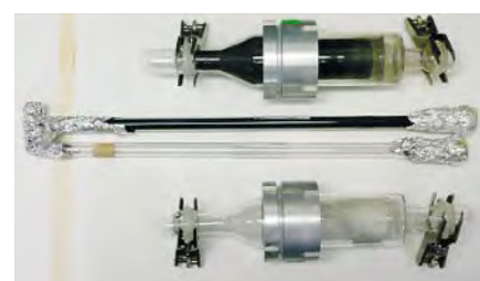
Fig. 2. Glass sampling devices exposed to 7 m 3 exhausts of a heavy duty engine (3 min operation) with and without filter.
