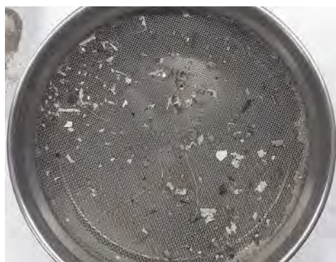
Sieve with particles >1 mm from Swiss floodplain soils. Many of the particles are plastics, as confirmed by ATR-FTIR spectroscopy.
