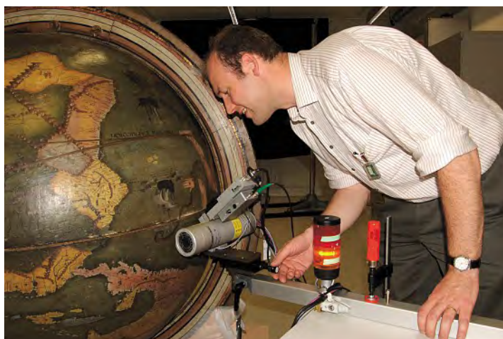
Setting up the XRF spectrometer for analysis
