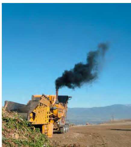
Fig. 1. Construction machinery in Switzerland has to be equipped with filters since 2009, but most trucks on roads are not.
