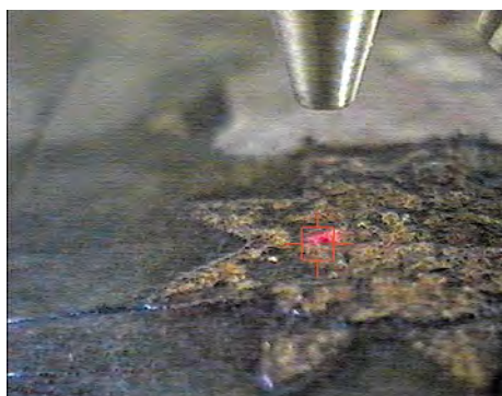
Focussing the X-ray beam on one of the gilded stars
