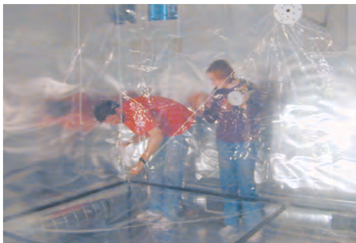
27 m 3 large smog chamber at PSI
